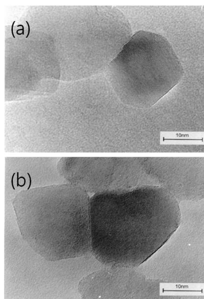
**Figure 1.** TEM images of  $\text{TiO}_2$  (a) and  $\text{WO}_3/\text{TiO}_2$  (b) nanoparticles.  $\text{TiO}_2$  is Degussa P25, and  $\text{WO}_3/\text{TiO}_2$  denotes to the surface-modified P25 with 3 mol% of  $\text{WO}_3$ .
