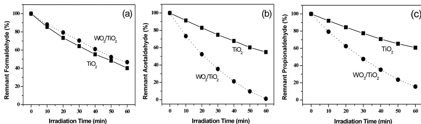
**Figure 2.** Percentage of remnant formaldehyde (a), acetaldehyde (b), and propionaldehyde (c) as a function of irradiation time by photocatalytic reaction with  $\text{TiO}_2$  and  $\text{WO}_3/\text{TiO}_2$ .
