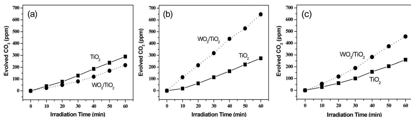
**Figure 3.** Evolution of  $\text{CO}_2$  from formaldehyde (a), acetaldehyde (b), and propionaldehyde (c) as a function of irradiation time with  $\text{TiO}_2$  and  $\text{WO}_3/\text{TiO}_2$  photocatalysts.
