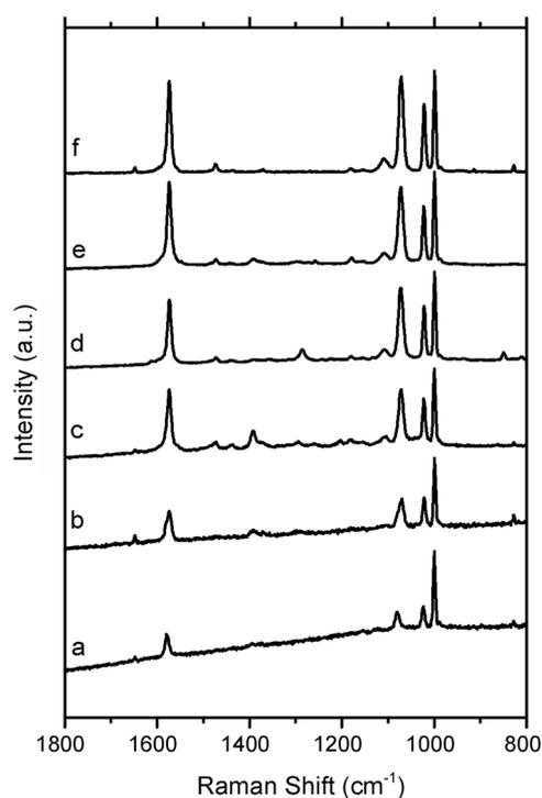
**Figure 3.** The typical SERS spectra of BT adsorbed on (a) pure  $\mu\text{Cu}$ , (b)  $\mu\text{Cu}@Ag(0.05)$ , (c)  $\mu\text{Cu}@Ag(0.5)$ , (d)  $\mu\text{Cu}@Ag(5)$ , (e)  $\mu\text{Cu}@Ag(50)$ , and (f) pure  $\mu\text{Ag}$  powders, respectively. All spectra were obtained using a He/Ne laser at 632.8 nm as the excitation source.
