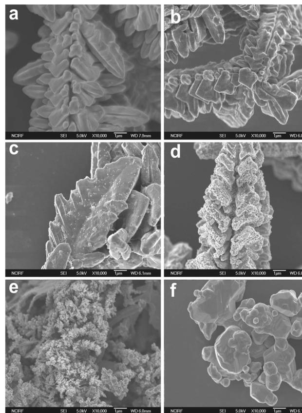
**Figure 1.** The typical FE-SEM images of (a) pure  $\mu\text{Cu}$ , (b)  $\mu\text{Cu}@Ag(0.05)$ , (c)  $\mu\text{Cu}@Ag(0.5)$ , (d)  $\mu\text{Cu}@Ag(5)$ , (e)  $\mu\text{Cu}@Ag(50)$ , and (f) pure  $\mu\text{Ag}$  powders.
