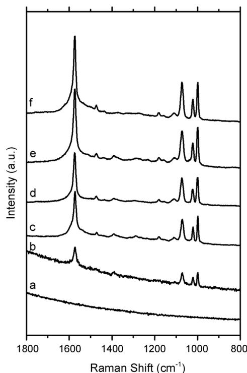
**Figure 5.** The typical SERS spectra of BT adsorbed on (a) pure  $\mu\text{Cu}$ , (b)  $\mu\text{Cu@Ag}(0.05)$ , (c)  $\mu\text{Cu@Ag}(0.5)$ , (d)  $\mu\text{Cu@Ag}(5)$ , (e)  $\mu\text{Cu@Ag}(50)$ , and (f) pure  $\mu\text{Ag}$  powders, respectively. All spectra were obtained using an  $\text{Ar}^+$  laser at  $514.5\text{ nm}$  as the excitation source.
