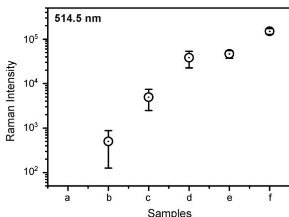
**Figure 6.** Relative Raman intensities of BT at 1574 cm<sup>-1</sup> adsorbed on (a) pure  $\mu\text{Cu}$ , (b)  $\mu\text{Cu@Ag}(0.05)$ , (c)  $\mu\text{Cu@Ag}(0.5)$ , (d)  $\mu\text{Cu@Ag}(5)$ , (e)  $\mu\text{Cu@Ag}(50)$  and (f) pure  $\mu\text{Ag}$  powders, respectively. Raman scattering intensities are the average of 5 measurements.
