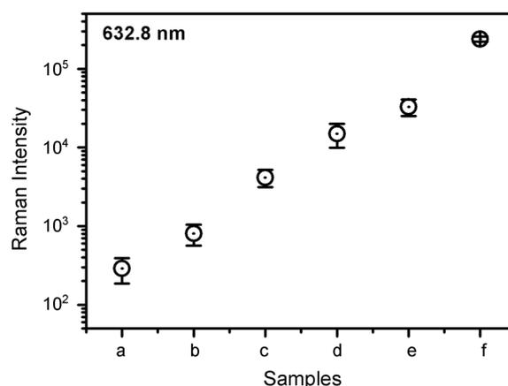
**Figure 4.** Relative Raman intensities of BT at  $1574\text{ cm}^{-1}$  adsorbed on (a) pure  $\mu\text{Cu}$ , (b)  $\mu\text{Cu@Ag}(0.05)$ , (c)  $\mu\text{Cu@Ag}(0.5)$ , (d)  $\mu\text{Cu@Ag}(5)$ , (e)  $\mu\text{Cu@Ag}(50)$  and (f) pure  $\mu\text{Ag}$  powders, respectively. Raman scattering intensities are the average of 5 measurements.
