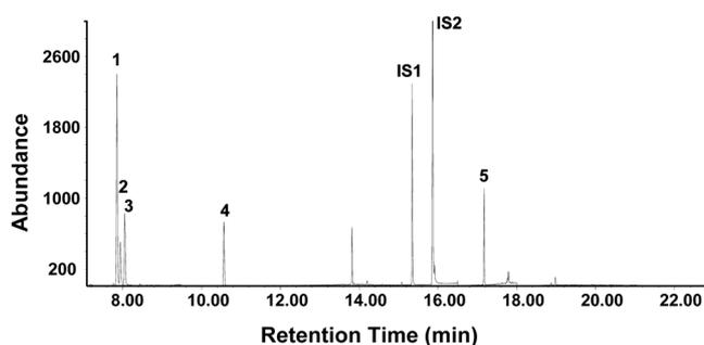
**Figure 5.** GC-MS-SIM chromatogram of chlorostyrenes in spiked fish sample at 10 ppb. Peak identities: 1. 4-chlorostyrene, 2. 2-chlorostyrene, 3. 3-chlorostyrene, 4. 2,6-dichlorostyrene, 5. octachlorostyrene, phenanthracene- $d_{10}$  (IS1) and  $^{13}\text{C}_6$ -HCB (IS2).
