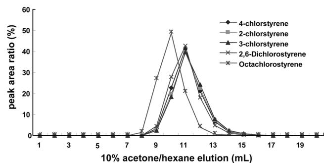
**Figure 3.** Elution patterns of chlorostyrenes on Florisil-SPE cartridge with acetone/*n*-hexane (1:9, v/v).
