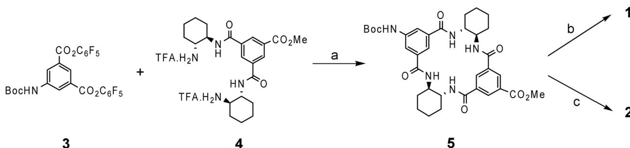
**Scheme 1.** Syntheses of metal-templated self-assembly (**1** and **2**); (a) slow addition to *i*Pr<sub>2</sub>NEt/THF. (b) TFA, then NEt<sub>3</sub>, bipyridine-carboxaldehyde and FeCl<sub>2</sub> in EtOH. (c) TFA, then NEt<sub>3</sub>, salicylaldehyde and FeCl<sub>3</sub> in EtOH.
