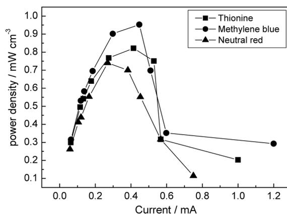
**Figure 3.** Polarization curves obtained when different mediators were used. Other conditions are the same as Fig. 2. Mediators ( $0.5 \text{ mM}$ ) are thionin (■), methylene Blue (●), and neutral Red (▲). Electrodeposition time was 5 min.
