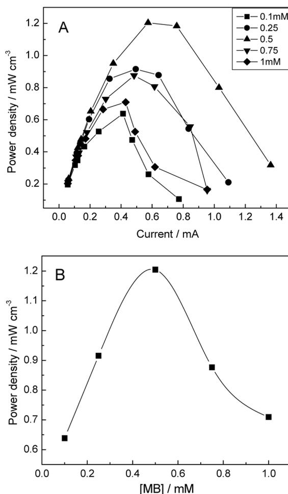
**Figure 4.** Polarization curves (A) and plot of power density vs. methylene Blue concentration (B). MB concentration are  $0.1 \text{ mM}$  (■),  $0.25 \text{ mM}$  (●),  $0.5 \text{ mM}$  (▲),  $0.75 \text{ mM}$  (▼), and  $1 \text{ mM}$  (◆). Other conditions are the same as Fig. 2. Electrodeposition time was 15 min.
