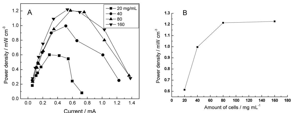
**Figure 5.** Polarization curves (A) obtained for different amount of bacterial cells: 20 mg mL<sup>-1</sup> (■), 40 mg mL<sup>-1</sup> (●), 80 mg mL<sup>-1</sup> (▲), and 160 mg mL<sup>-1</sup> (▼). Panel B was constructed from panel A. Other conditions are the same as Figure 2.
