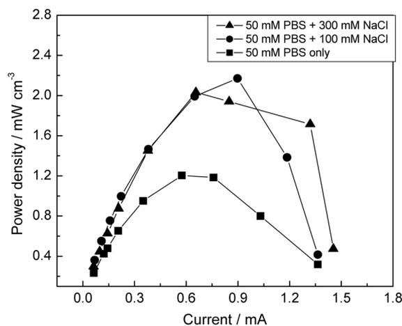
**Figure 6.** Polarization curves obtained for different ionic strength of NaCl: No NaCl (■), 100 mM (●), 300 mM (▲). *P. vulgaris*: 80 mg mL<sup>-1</sup>. Phosphate buffer concentration was maintained at 50 mM. Other conditions are the same as Figure 2.
