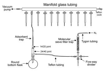
Figure 2. Scheme of solid-phase tapping-solvent extraction (SPTE) apparatus.
