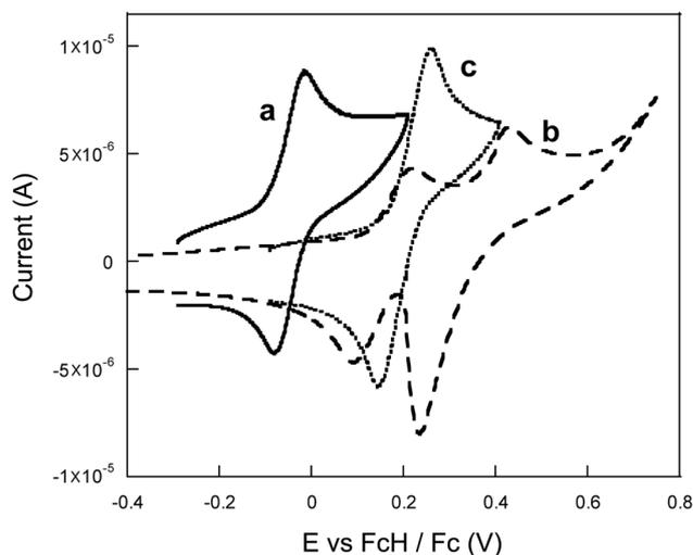
**Figure 3.** Cyclic voltammograms of **1N** (a), **2N** (b) and **3N** (c). CV was carried out relative to ferrocene in 0.1 M *n*-Bu<sub>4</sub>NPF<sub>6</sub> in THF with a scan rate of 100 mV/s.
