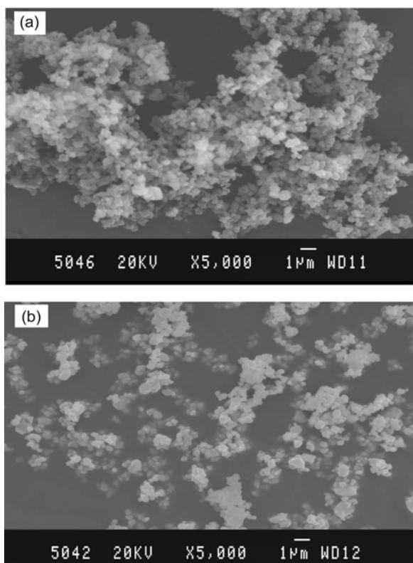
**Figure 3.** Scanning electron micrographs of (a) pure PPy and (b) PPy/PbTiO<sub>3</sub> (50 wt %).
