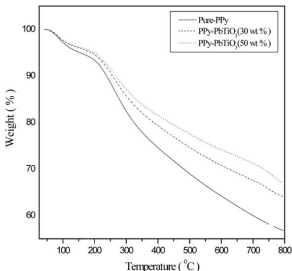
**Figure 4.** TGA curves obtained from PPy, PPy/PbTiO<sub>3</sub> (30 wt %), and PPy/PbTiO<sub>3</sub> (50 wt %).
