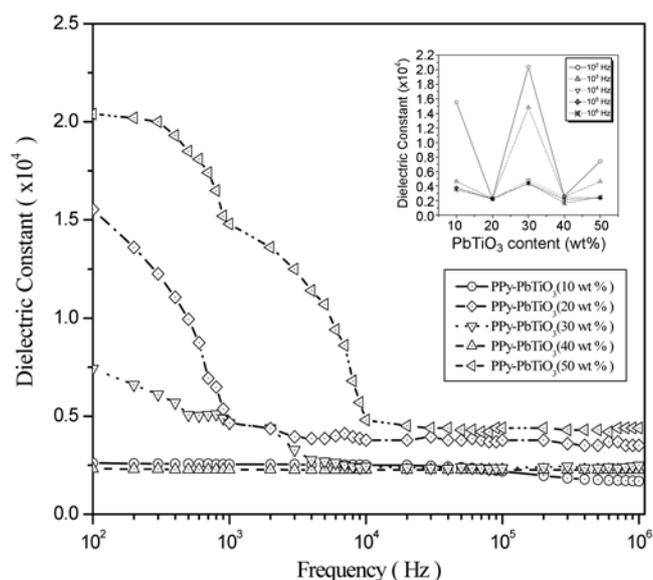
**Figure 6.** Frequency-dependent dielectric constant of PPy/ $\text{PbTiO}_3$  composites (Inset: Dielectric constant of PPy/ $\text{PbTiO}_3$  composites for different wt % of  $\text{PbTiO}_3$  at different frequencies).
