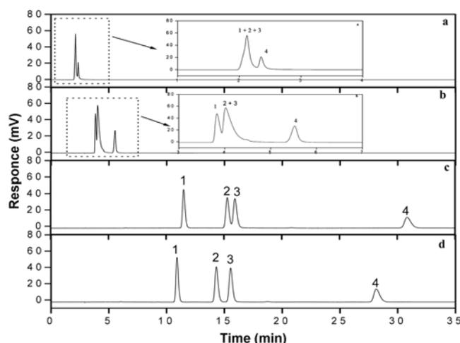
**Figure 2.** Chromatograms of a mixture of nucleotides with mobile phases without (a) and with 0.5 (b), 10.0 (c) and 13.0 (d) mM [BMIm][BF<sub>4</sub>] (peaks numbering: (1) 5'-UMP, (2) 5'-IMP, (3) 5'-GMP, (4) 5'-TMP).
