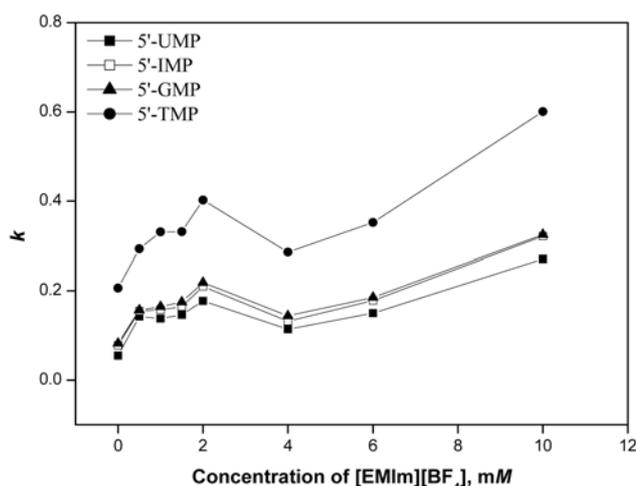
**Figure 3.** Retention factors ( $k$ ) of nucleotides without and with [EMIm][BF<sub>4</sub>] in mobile phase.
