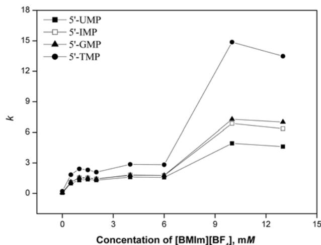
**Figure 1.** Retention factors ( $k$ ) of nucleotides without and with [BMIm][BF<sub>4</sub>] in mobile phase.
