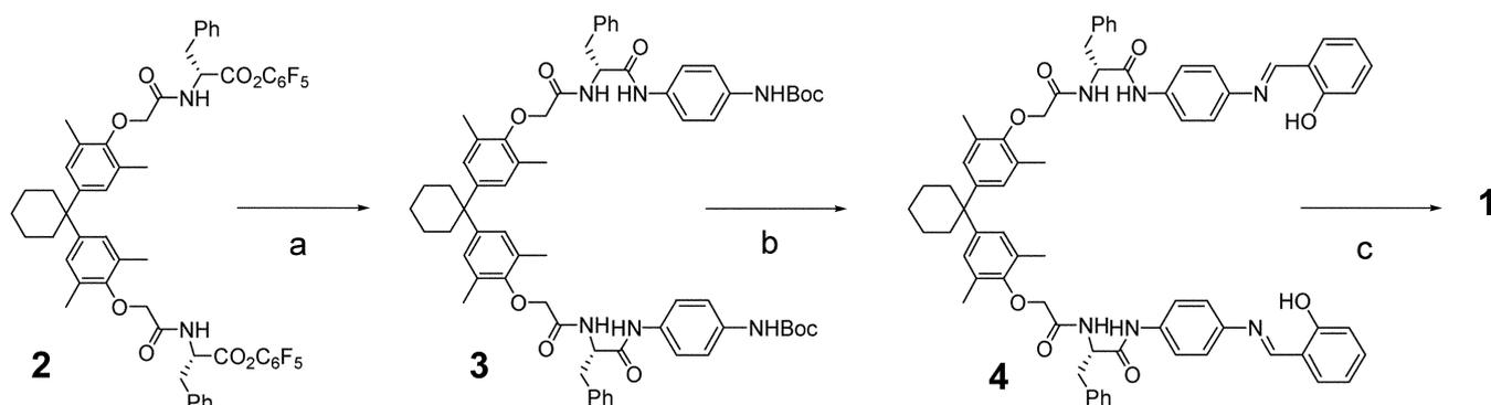
**Scheme 1.** Synthesis of Metallomacrocyclic (**1**); (a) mono-Boc-1,4-phenylene diamine. (b) TFA, then salicylic aldehyde in EtOH. (c) FeCl<sub>3</sub>.
