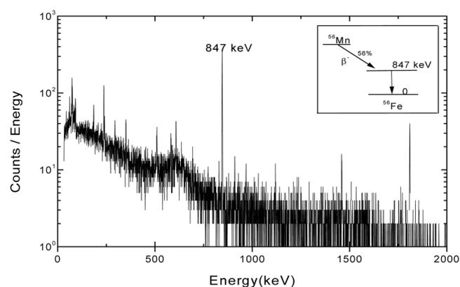
**Figure 4.** Gamma ray pulse height spectrum by <sup>55</sup>Mn(n,  $\gamma$ )<sup>56</sup>Mn reaction.
