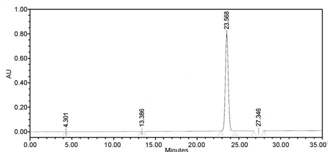
**Figure 4.** HPLC-PDA chromatogram of QN09 (Wavelength 266 nm). Column: Luna C<sub>18</sub>, 4.6 mm × 250 mm, 5 μm; mobile phase: MeCN: water: TFA (34 : 66 : 0.1, v:v:v); detector wavelength: 266 nm; flow rate: 1.0 mL/min; Temperature: 30 °C
