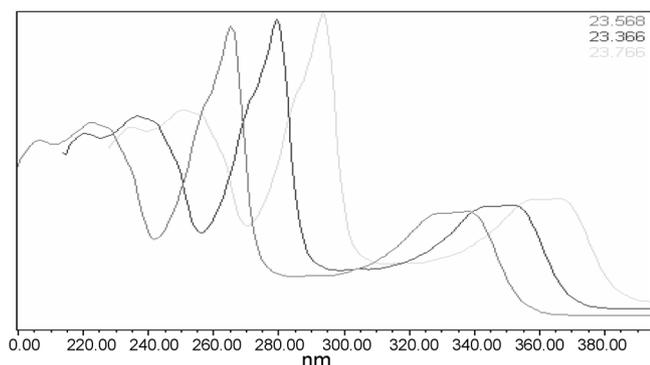
**Figure 5.** UV spectra for the apex and two points corresponding to half the height of the peak for QN09.
