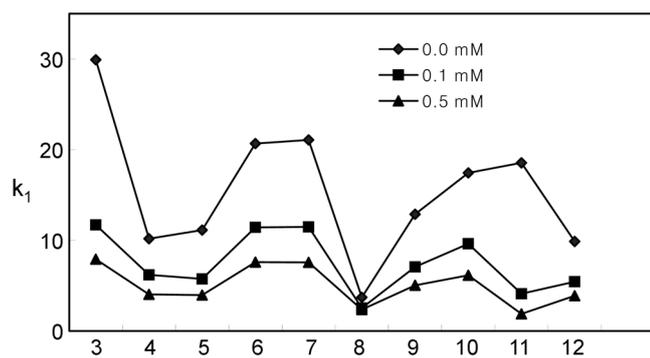
**Figure 3.** The trends of the retention factors ( $k_1$ ) for the resolution of  $\beta$ -amino acids 3-12 on CSP 2 with the variation of the ammonium acetate ( $\text{NH}_4\text{OAc}$ ) concentration (0.0 mM, 0.1 mM and 0.5 mM) in aqueous mobile phase.
