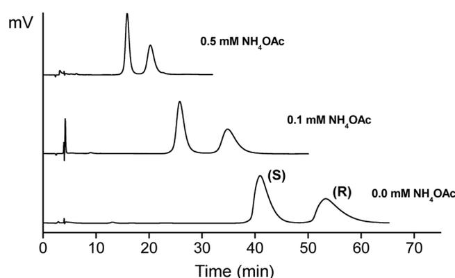
**Figure 5.** The representative chromatograms for the resolution of 3-amino-4-(4-methylphenyl)butyric acid (**4**) on CSP 2 with the variation of the ammonium acetate ( $\text{NH}_4\text{OAc}$ ) concentration (0.0 mM, 0.1 mM and 0.5 mM) in aqueous mobile phase. For the chromatographic condition, see the foot note to Table 2.
