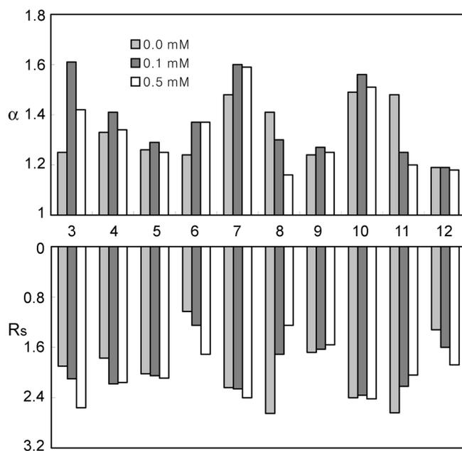
**Figure 4.** The trends of the separation ( $\alpha$ ) and the resolution factors ( $R_s$ ) for the resolution of  $\beta$ -amino acids 3-12 on CSP 2 with the variation of the ammonium acetate ( $\text{NH}_4\text{OAc}$ ) concentration (0.0 mM, 0.1 mM and 0.5 mM) in aqueous mobile phase.
