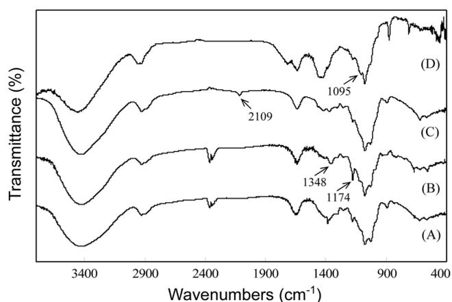
**Figure 3.** FTIR spectra of neutral cyclophorases (A) and their derivatives. Tosyl-cyclophorases (B), azido-cyclophorases (C), amino-cyclophorases (D). Spectra were acquired between 4000 and 400  $\text{cm}^{-1}$ .
