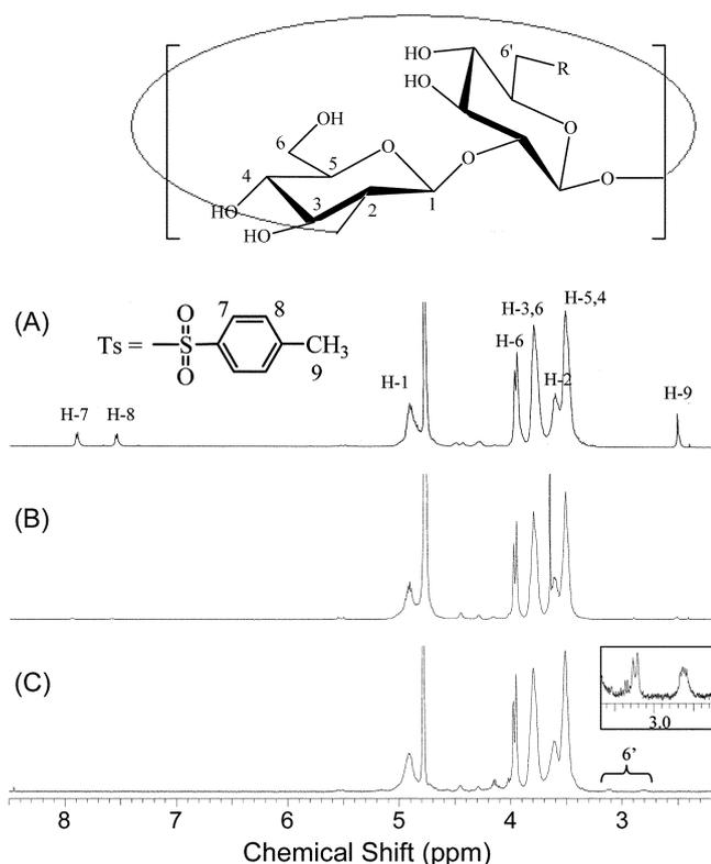
**Figure 2.**  $^1\text{H}$  NMR spectra of cyclophorases derivatives. Tosyl-cyclophorases (A), azido-cyclophorases (B), amino-cyclophorases (C).
