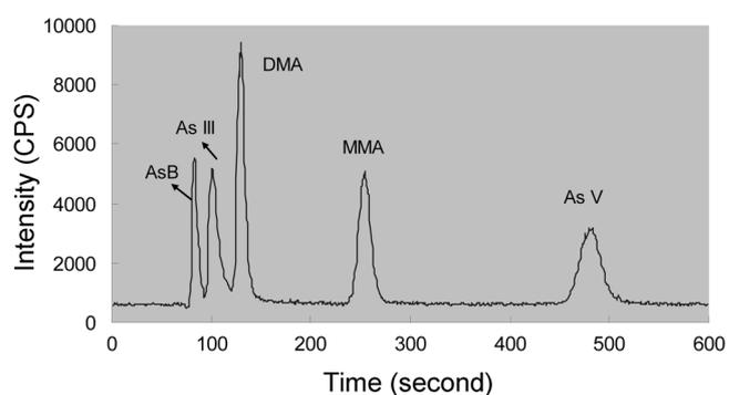
**Figure 1.** HPLC-ICP-MS chromatogram of standard containing 10  $\mu\text{g/L}$  each of As(III), As(V), MMA, DMA, and AsB.
