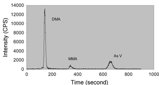
**Figure 3.** HPLC-ICP-MS chromatogram of arsenic species in rice flour SRM 1568a.
