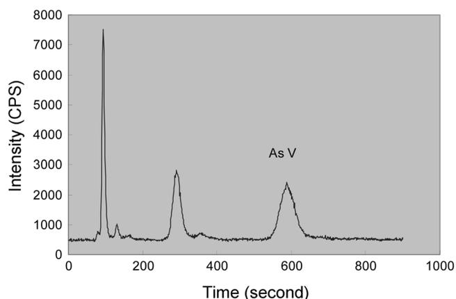
**Figure 7.** HPLC-ICP-MS chromatogram of arsenic species in an herbal dietary supplement (sample 3) with enzyme extraction.
