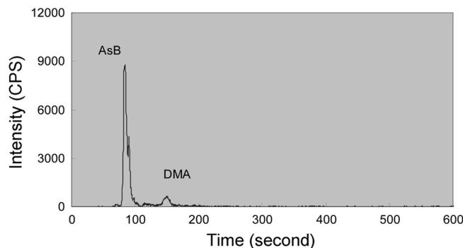
**Figure 4.** HPLC-ICP-MS chromatogram of arsenic species in tuna fish tissue BCR-627.
