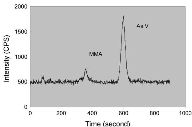
**Figure 6.** HPLC-ICP-MS chromatogram of arsenic species in an herbal dietary supplement (sample 2) with enzyme extraction.
