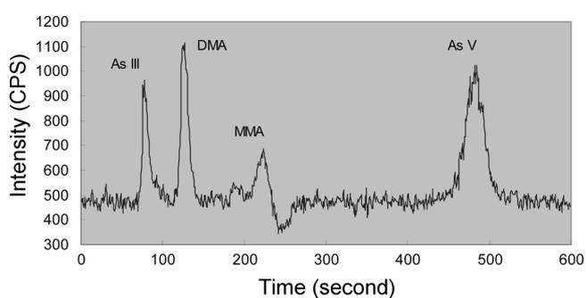
**Figure 2.** HPLC-ICP-MS chromatogram of arsenic species in a freeze-dried apple sample.
