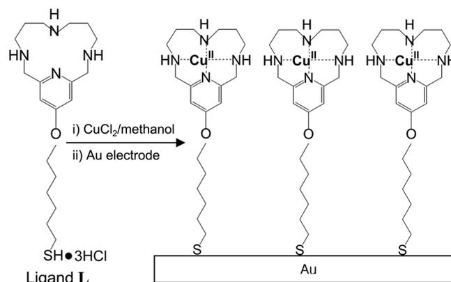
**Figure 1.** Molecular structure of the ligand **L** and formation of the electroactive self-assembled monolayer consisted of Cu(II) complex of **L** on Gold thin film electrode.
