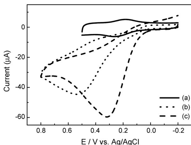
**Figure 2.** Typical cyclic voltammograms of (a) Au electrode modified with SAM of CuL complex in 0.1 M phosphate buffer (pH 7.01), (b) bare Au electrode and (c) Au electrode modified with SAM of CuL complex in 0.1 M phosphate buffer solution (pH 7.01) containing 1.0 mM ascorbic acid. All scan rates were 100 mV/s.
