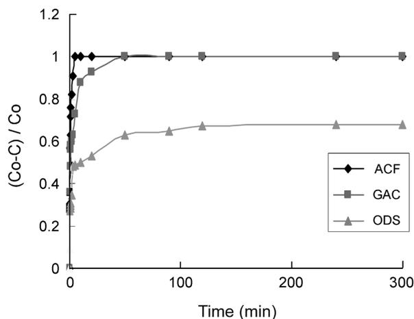
**Figure 2.** The time dependent adsorption behaviours of microcystin LR onto three different adsorbents (ACF, GAC and ODS).
