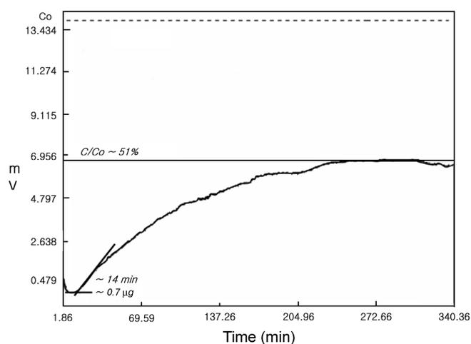
**Figure 3.** Breakthrough Curve of Microcystin LR over ACF ACF was NPV 10400 (0.6 mg), adsorbate was microcystin LR (1 μg/mL) and flow rate was 0.05 mL/min.
