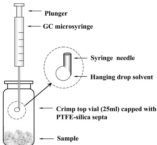
**Figure 1.** Schematic diagram of headspace hanging drop liquid phase microextraction (HS-HD-LPME).
