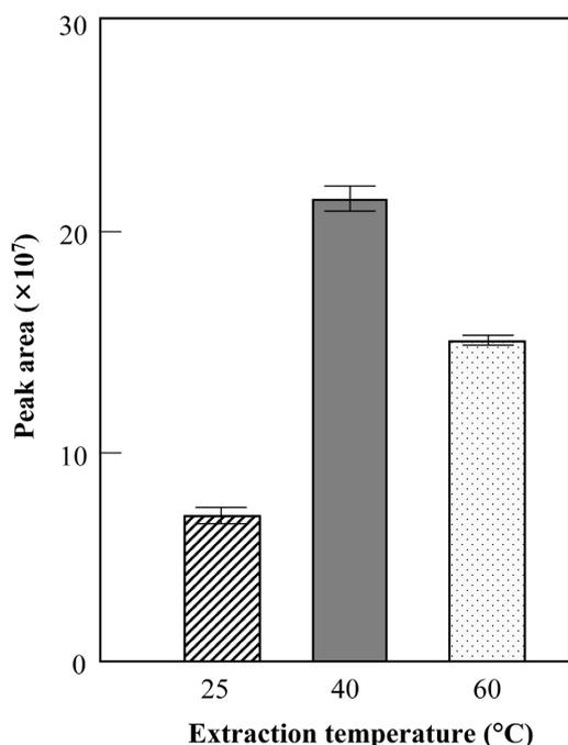
**Figure 2.** Effect of extraction temperature on the analytical signal for linalool in HS-HD-LPME.
