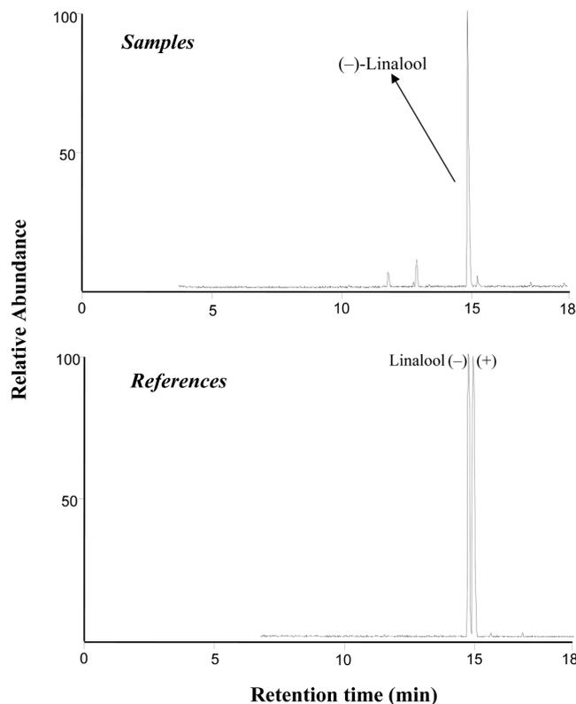
**Figure 5.** Enantiomeric separations of linalool isolated from evening primrose flowers using a 30% heptakis (2,3-di-O-methyl-6-O-*t*-butyldimethyl-silyl)- $\beta$ -cyclodextrin (Cyclosil-B, J&W, 30 m  $\times$  0.25 mm  $\times$  0.25  $\mu\text{m}$  film thickness) column.
