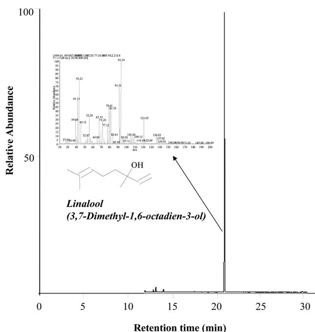
**Figure 4.** Total ion chromatogram and mass spectra (inset) of linalool obtained by HS-HD-LPME from evening primrose flowers sample.
