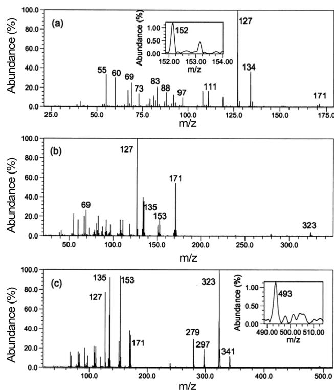
**Figure 2.** Variation of the mass spectra of cyclohexane butyric acid with the ion trapping time. The electron impact energy is 50 eV. The sample pressures and ion trapping times are  $1.6 \times 10^{-6}$  Torr/1 ms (a),  $2.1 \times 10^{-6}$  Torr/50 ms (b), and  $3.6 \times 10^{-6}$  Torr/200 ms (c).
