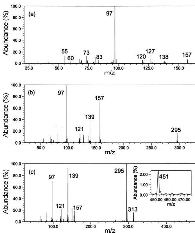
**Figure 1.** Variation of the mass spectra of cyclohexane propionic acid with the ion trapping time. The electron impact energy is 50 eV. The sample pressures and ion trapping times are  $4.0 \times 10^{-6}$  Torr/1 ms (a),  $3.0 \times 10^{-6}$  Torr/50 ms (b), and  $2.5 \times 10^{-6}$  Torr/300 ms (c).
