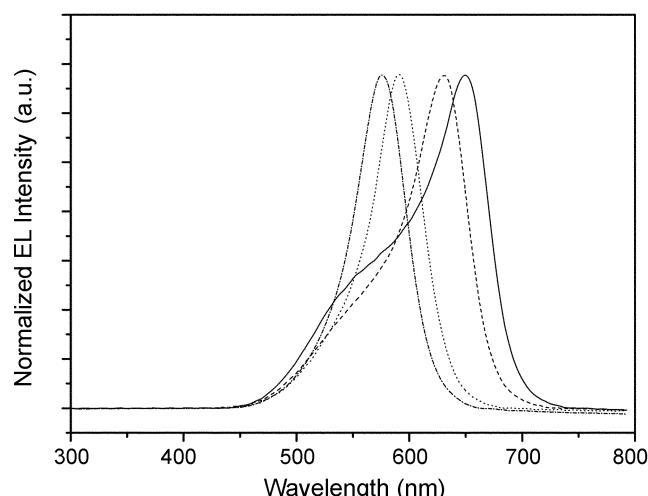
**Figure 2.** Normalized EL spectra of green device,  $\text{Al}(200 \text{ nm})/2\text{-TNATA}(60 \text{ nm})/\text{NPB}(15 \text{ nm})/\text{Alq}_3(70 \text{ nm})/\text{LiF}(1 \text{ nm})/\text{Al}(20 \text{ nm})$ . Detection angle: (—):  $0^\circ$ , (---):  $30^\circ$ , (···):  $60^\circ$ , (····):  $90^\circ$ .
