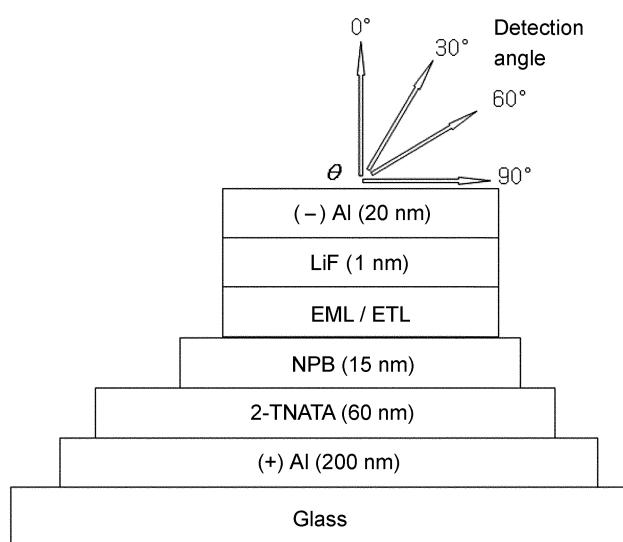
**Figure 1.** Configuration and detection angle of devices. EML/ETL thickness: green ( $\text{Alq}_3$  70 nm), red ( $(\text{Alq}_3 + 3\% \text{ DCM2})$  30 nm/ $\text{Alq}_3$  30 nm), blue ( $\text{DPVBi}$  30 nm/ $\text{Alq}_3$  30 nm).
