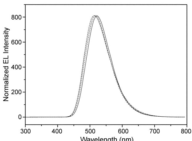
**Figure 3.** Normalized EL spectra of conventional green device,  $\text{ITO}/2\text{-TNATA}(60 \text{ nm})/\text{NPB}(15 \text{ nm})/\text{Alq}_3(70 \text{ nm})/\text{LiF}(1 \text{ nm})/\text{Al}(20 \text{ nm})$ . Detection angle: (—):  $0^\circ$ , (---):  $30^\circ$ , (···):  $60^\circ$ , (····):  $90^\circ$ .
