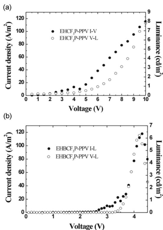
**Figure 5.** Current-voltage-luminescence (I-V-L) characteristics of PLEDs of EHCF<sub>3</sub>P-PPV and EHBCF<sub>3</sub>P-PPV with a configuration of ITO/PEDOT:PSS/polymer/Al.
