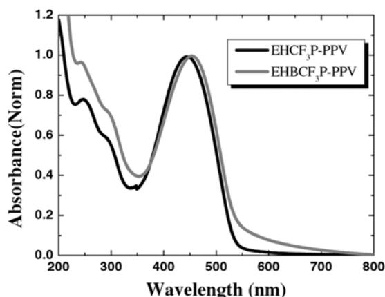
**Figure 1.** UV-vis absorption spectra of  $\text{EHCF}_3\text{P-PPV}$  and  $\text{EHBCF}_3\text{P-PPV}$ .
