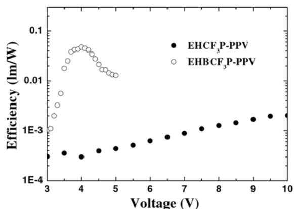
**Figure 6.** Efficiencies of PLEDs of EHCF<sub>3</sub>P-PPV and EHBCF<sub>3</sub>P-PPV with a configuration of ITO/PEDOT:PSS/polymer/Al.
