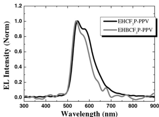
**Figure 4.** Electroluminescence spectra of EHCF<sub>3</sub>P-PPV and EHBCF<sub>3</sub>P-PPV.
