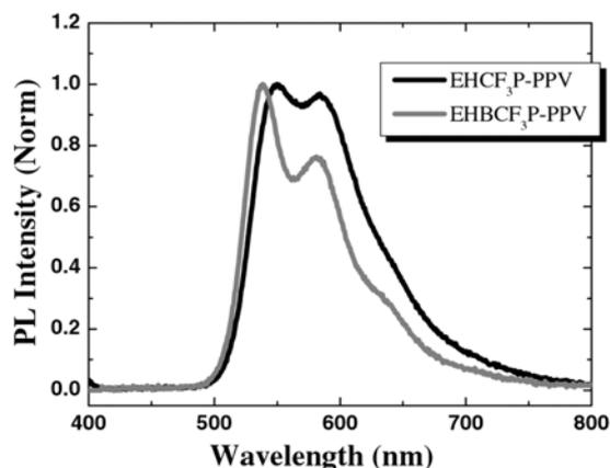
**Figure 2.** Photoluminescence spectra of  $\text{EHCF}_3\text{P-PPV}$  and  $\text{EHBCF}_3\text{P-PPV}$ .
