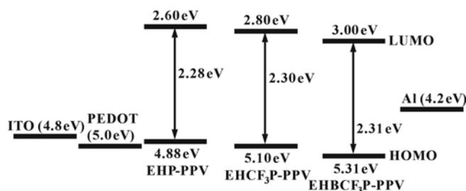
**Figure 3.** Energy band diagram of EHCF<sub>3</sub>P-PPV and EHBCF<sub>3</sub>P-PPV.
