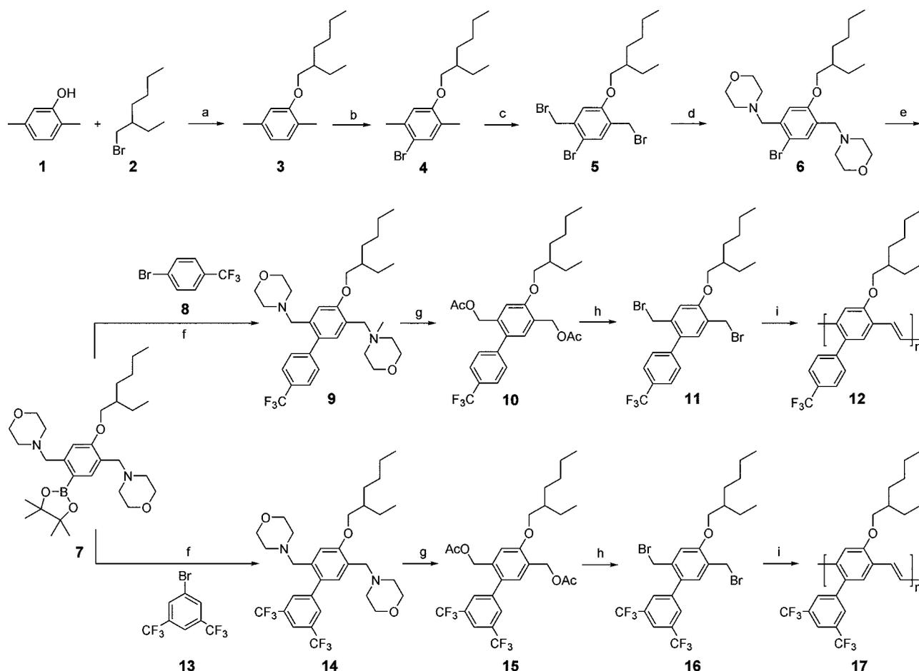
**Scheme 1.** (a) KOH, EtOH, reflux; (b) NBS, DMF; (c) NBS (2eq), CCl<sub>4</sub>; (d) Morpholine, EtN(*i*-Pr)<sub>2</sub>, THF; (e) 2-isopropoxy-4,4,5,5-tetramethyl-1,3,2-dioxaborolane, *n*-BuLi, THF, -78 °C; (f) Pd(PPh<sub>3</sub>)<sub>4</sub>, Na<sub>2</sub>CO<sub>3</sub>, DME, H<sub>2</sub>O; (g) Ac<sub>2</sub>O, reflux; (h) HBr, CH<sub>2</sub>Cl<sub>2</sub>; (i) *tert*-BuOK, THF.
