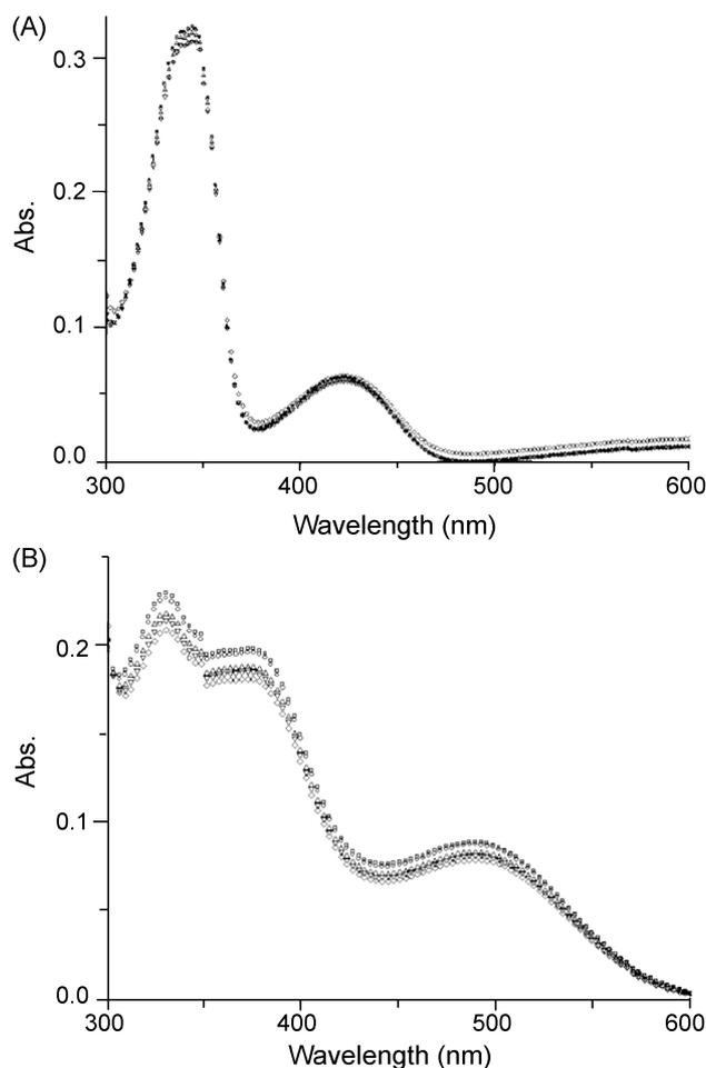
**Figure 5.** Influence of DNA binding on the visible absorption spectra of berberine (A) and berberrubine (B). Fixed concentrations of drug were titrated with increasing concentrations of HP14. Drug concentrations were maintained below  $5 \mu\text{M}$  throughout the experiment.
