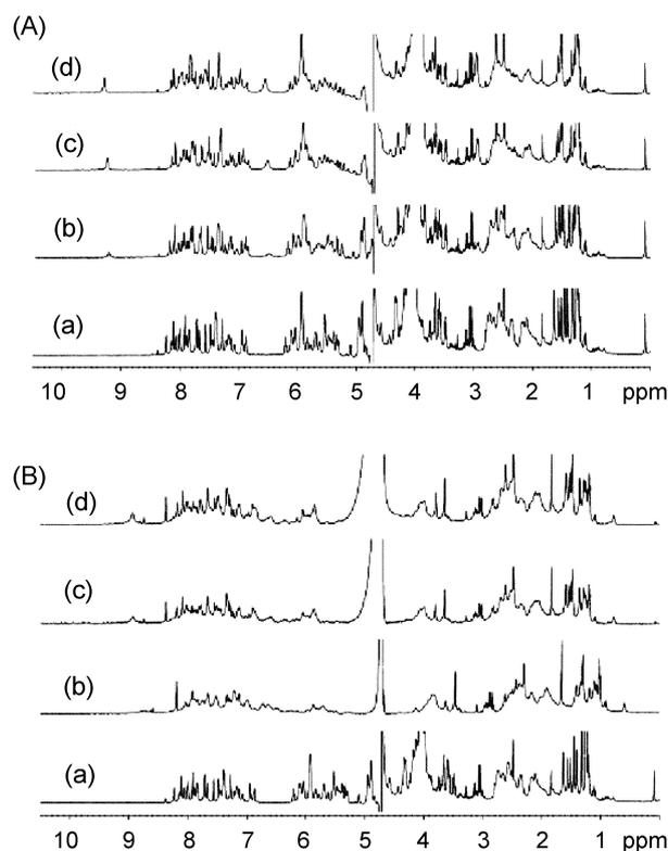
**Figure 2.** The aliphatic proton region of 1D-<sup>1</sup>H NMR spectra of berberine/HP14 complex (A) and berberrubine/HP14 complex (B) acquired at 25 °C in 100 mM KCl, 50 mM phosphate buffer and pH 7.0 in D<sub>2</sub>O. The molar ratio between HP14 and berberine is (a) 1 : 0. (b) 1 : 1. (c) 1 : 3. (d) 1 : 6.
