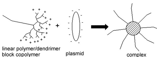
**Scheme 1.** Schematic view of the formation of self-assembling complexes. The polyionic complexes are coated with hydrophilic PEG chains.
