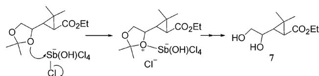
**Scheme 2.** Proposed mechanism for a Lewis acid induced deketalisation.silyl ether **10** with HCl to **11** (entry 3c versus 1c and 2c).
