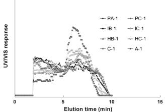
**Figure 4**. Power-programmed Sd/StFFF fractograms of Group-1 airborne samples. The experimental conditions were the same as those in Figure 3.
