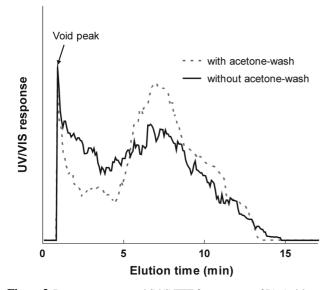
**Figure 3**. Power-programmed Sd/StFFF fractograms of IA-1 airborne sample with and without acetone-washing. The programming parameters were: initial field strength = 300 rpm,  $t_a = 4$ ,  $t_i = -16$ , and p = 8. The flow rate was 7 mL/min.
