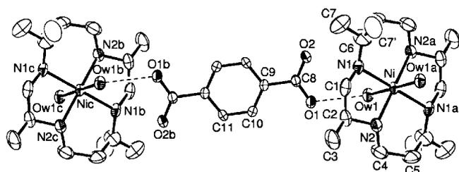
**Figure 1.** An ORTEP drawing of  $[\text{Ni}(\text{L})(\text{H}_2\text{O})_2](\text{tp})\cdot 4\text{H}_2\text{O}$  (**1**) with the atomic numbering scheme (30% probability ellipsoids shown).
