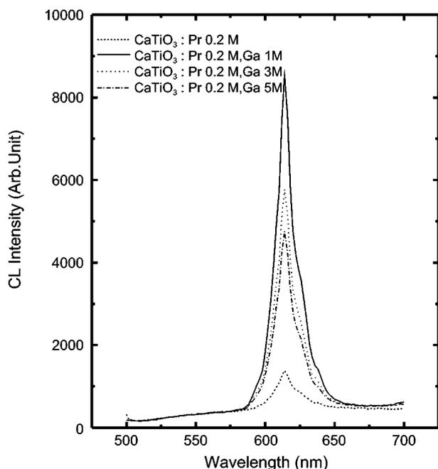
**Figure 2.** CL intensity of  $\text{Ga}(x)$ -doped  $\text{CaTiO}_3:\text{Pr}$  ( $x = 1, 2, 3$  mole %). (anode voltage and current: 1 kV, 20  $\mu\text{A}$ )
