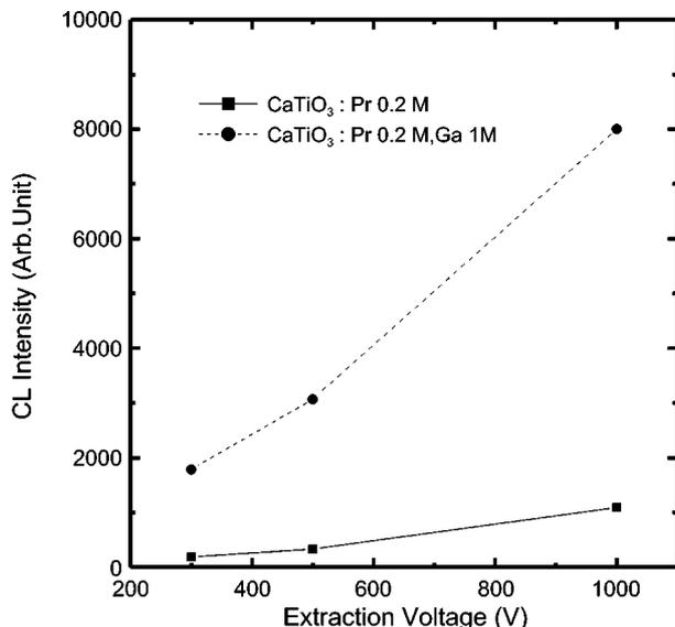
**Figure 4.** Maximal peak CL intensities at 614 nm of CaTiO<sub>3</sub>:Pr (0.2%), Ga (1%) and CaTiO<sub>3</sub>:Pr (0.2%) with various anode voltages. (anode current: 20  $\mu$ A)
