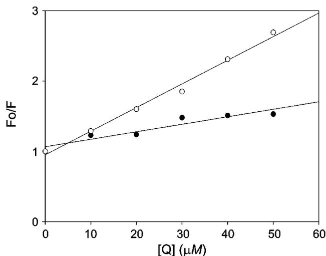
**Figure 3.** Plot of  $F_0/F$  vs  $[Q]$  according to Stern-Volmer equation in aqueous medium with safranin O ( $\circ$ ) and thionin ( $\bullet$ ). Calculated Stern-Volmer quenching constants ( $K_{SV}$ ) of mediators are  $0.0336 \text{ M}^{-1}$  for safranin O and  $0.0107 \text{ M}^{-1}$  for thionin.
