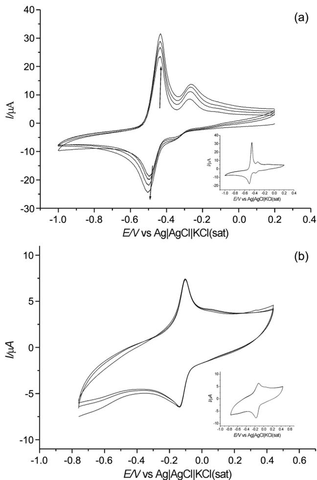
**Figure 2.** Cyclic voltammograms of safranin O (a) and thionin (b) in the PC film at pH 7.0 solution. Scan rate:  $100 \text{ mV}\cdot\text{s}^{-1}$ ; Electrode area:  $0.071 \text{ cm}^2$ . Inset shows the voltammogram on the bare electrode.
