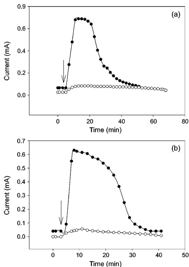
**Figure 1.** Variation of current output with time through the 560- $\Omega$  external load for fuel cells containing (a) *P. vulgaris* and (b) *E. coli* with safranin O (○) and thionin (●) as the electron transfer mediator. Organism concentration: 1 mg (dry wt) mL<sup>-1</sup>; 1  $\mu\text{mol}$  of mediator and 1  $\mu\text{mol}$  of glucose were added. Addition of glucose is marked by the arrows.
