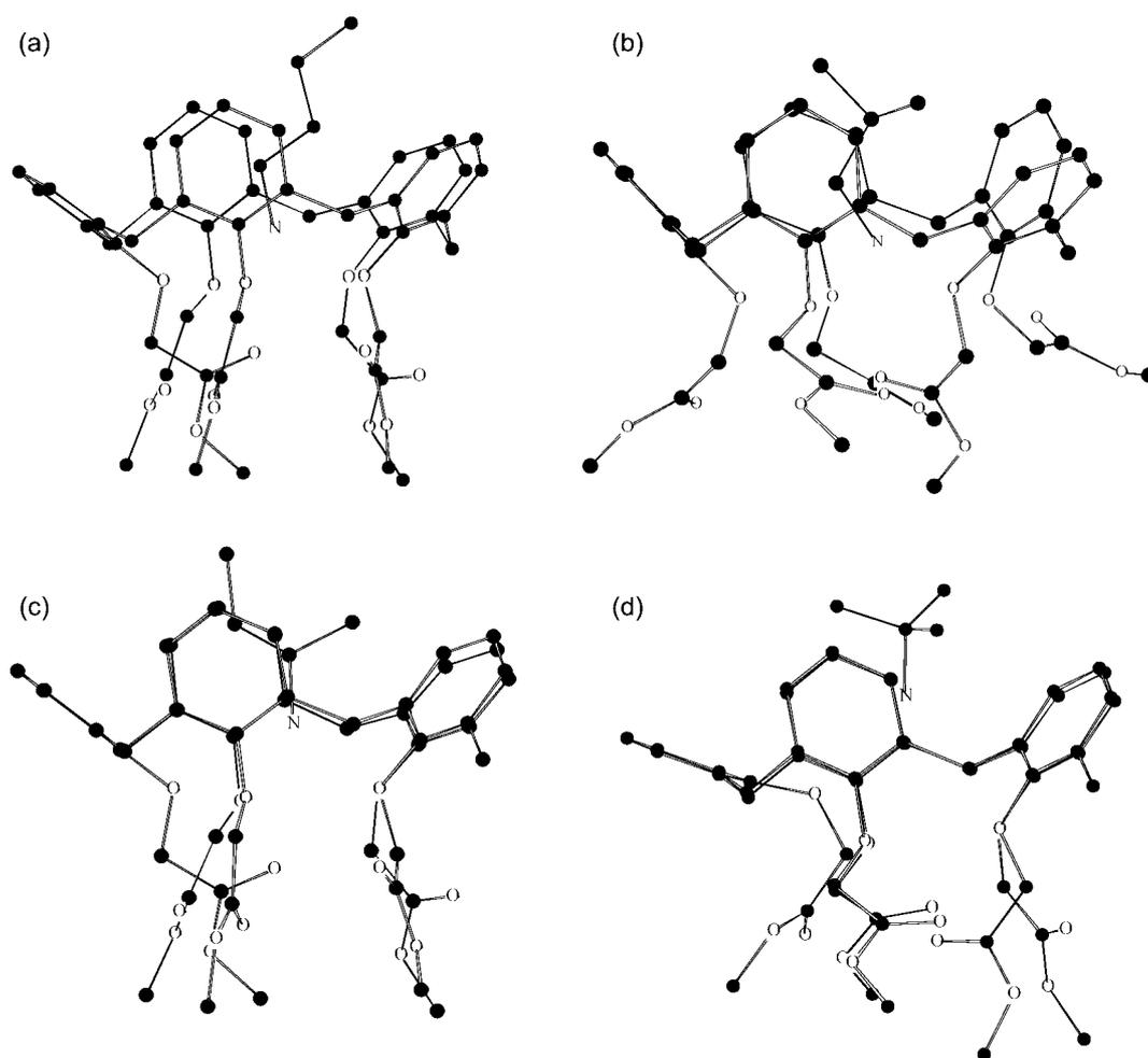
**Figure 6.** *Ab initio* calculated *endo*-cone conformations of **2e** complexed with (a) *n*-butyl ammonium, (b) *iso*-butyl ammonium, (c) *sec*-butyl ammonium, and (d) *tert*-butyl ammonium ions.
