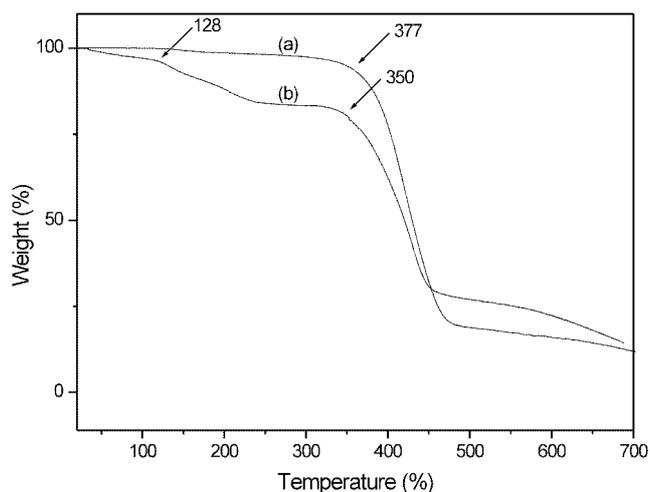
**Figure 3.** TGA thermograms of (a) poly(ST-co-VBC) and (b) poly(ST-co-VBC)-DMAP. The scanning rate was 20 °C/min.
