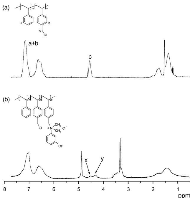
**Figure 2.** <sup>1</sup>H NMR spectra of (a) poly(ST-co-VBC) (CDCl<sub>3</sub>) and (b) poly(ST-co-VBC)-DMAP (CD<sub>3</sub>OD).
