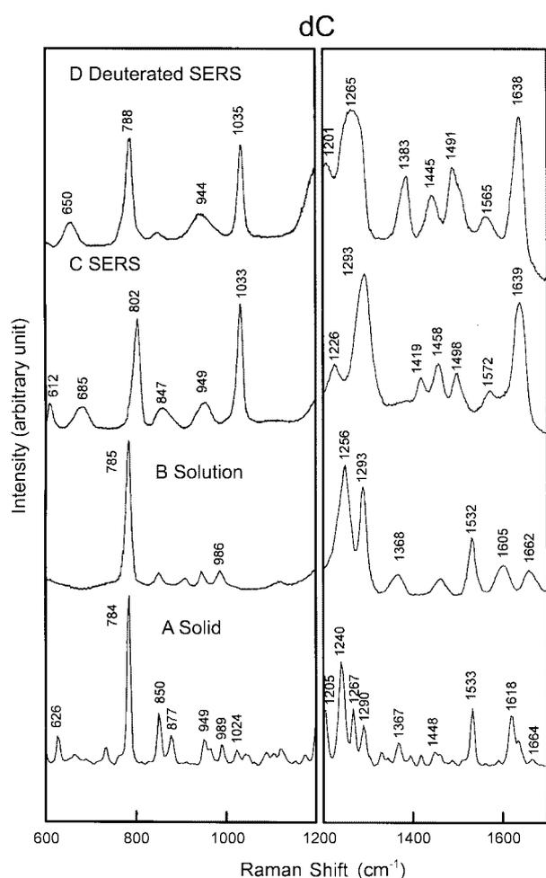
**Figure 4.** The Raman spectra as in Figure 3 of dC. The spectra of (a) and (b) have been subtracted by baseline.
