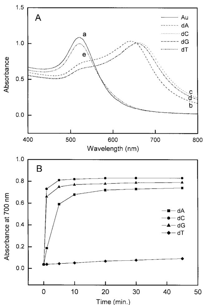
**Figure 2.** UV-Visible absorption spectra of a gold nanoparticles: (A) (a) in the absence of adsorbate and 5 minutes after modifying with DNA nucleosides (b) dA (c) dC (d) dG, and (e) dT; (B) depending on time after modification at 700 nm for (f) dA, (g) dC, (h) dG, and (i) dT.
