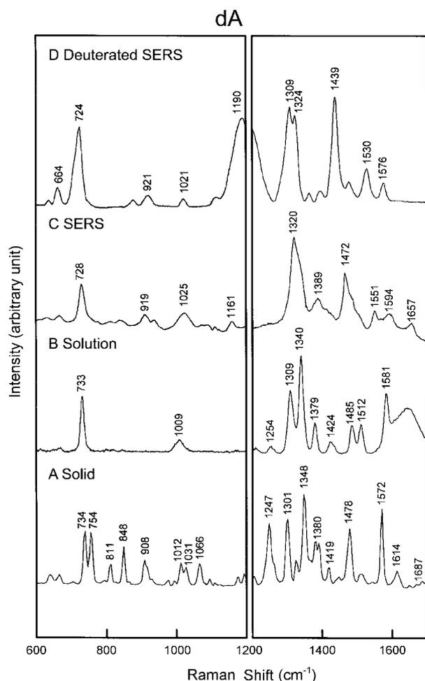
**Figure 3.** The Raman spectra of dA: (a) FT-Raman in solid, (b) Normal Raman in aqueous solution (saturated), (c) SERS on aqueous gold nanoparticles ( $1.5 \times 10^{-5}$  M), (d) SERS on gold nanoparticles in  $D_2O$  for N-Deuterated species ( $1.5 \times 10^{-5}$  M). The laser power and excitation wavelength is (a) 200 mW with 1064 nm Nd:YAG, (b) 200 mW with 488 nm  $Ar^+$ , (c) and (d) 100 mw with 710 nm  $Ti:Al_2O_3$  prism pumped  $Ar^+$  laser.
