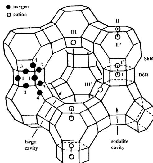
**Figure 1.** A stylized drawing of the framework structure of zeolite X. Near the center of each line segment is an oxygen atom. The different oxygen atoms are indicated by the numbers 1 to 4. Silicon and aluminum atoms alternate at the tetrahedral intersections, except that Si substitutes for about 4% of the Al atoms. Extraframework cation positions are labeled with Roman numerals.
