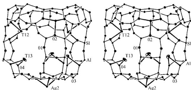
**Figure 4.** Stereoview of a supercage in dehydrated  $\text{Ag}_{27}\text{Tl}_{65}\text{-X}$ . Two  $\text{Ag}^+$  ions at Ag(2) (site II'), two  $\text{Tl}^+$  ions at Tl(2) (site II) and three  $\text{Tl}^+$  ions at Tl(3) (site III') are shown. About 50% of supercages may have an arrangement like this. Ellipsoids of 20% probability are used.
