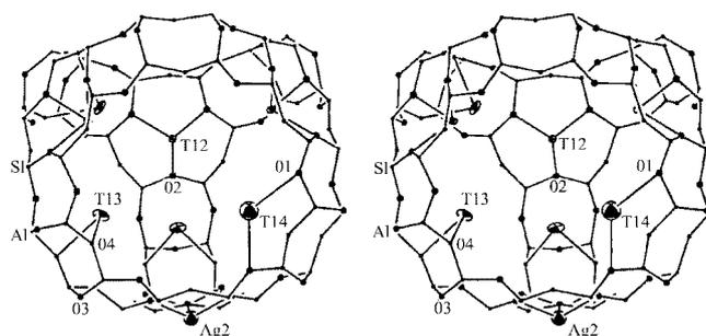
**Figure 6.** Stereoview of a supercage of dehydrated  $\text{Ag}_{23}\text{Tl}_{69}\text{-X}$ . One  $\text{Ag}^+$  ion at Ag(2) (site II'), three  $\text{Tl}^+$  ions at Tl(2) (site II), three  $\text{Tl}^+$  ions at Tl(3) (site III') and one  $\text{Tl}^+$  ion at Tl(4) (site III') are shown. About 50% of supercages may have this arrangement. Ellipsoids of 20% probability are used.
