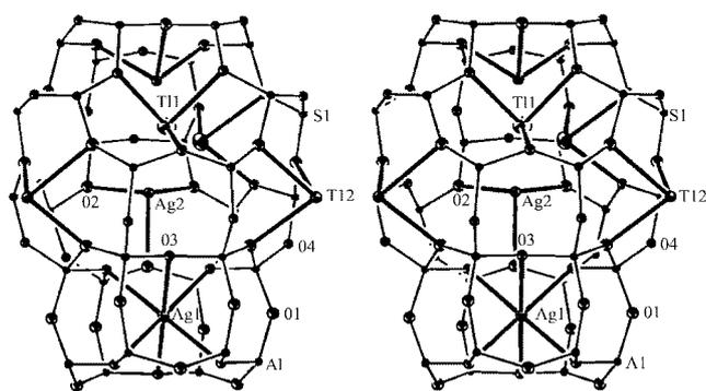
**Figure 3.** Stereoview of a sodalite cavity with an attached D6R in dehydrated  $\text{Ag}_{27}\text{Tl}_{65}\text{-X}$ . One  $\text{Ag}^+$  ion at Ag(1) (site I), two  $\text{Ag}^+$  ions at Ag(2) (site II'), two  $\text{Tl}^+$  ions at Tl(1) (site I') and two  $\text{Tl}^+$  ions at Tl(2) (site II) are shown. About 50% of sodalite cavities may have this arrangement. Ellipsoids of 20% probability are used.
