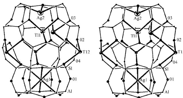
**Figure 5.** Stereoview of a sodalite cavity with an attached D6R in dehydrated  $\text{Ag}_{23}\text{Tl}_{69}\text{-X}$ . One  $\text{Ag}^+$  ion at Ag(1) (site I), one  $\text{Ag}^+$  ion at Ag(2) (site II'), two  $\text{Tl}^+$  ions at Tl(1) (site I') and three  $\text{Tl}^+$  ions at Tl(2) (site II) are shown. About 87.5% of sodalite cavities may have this arrangement. Ellipsoids of 20% probability are used.
