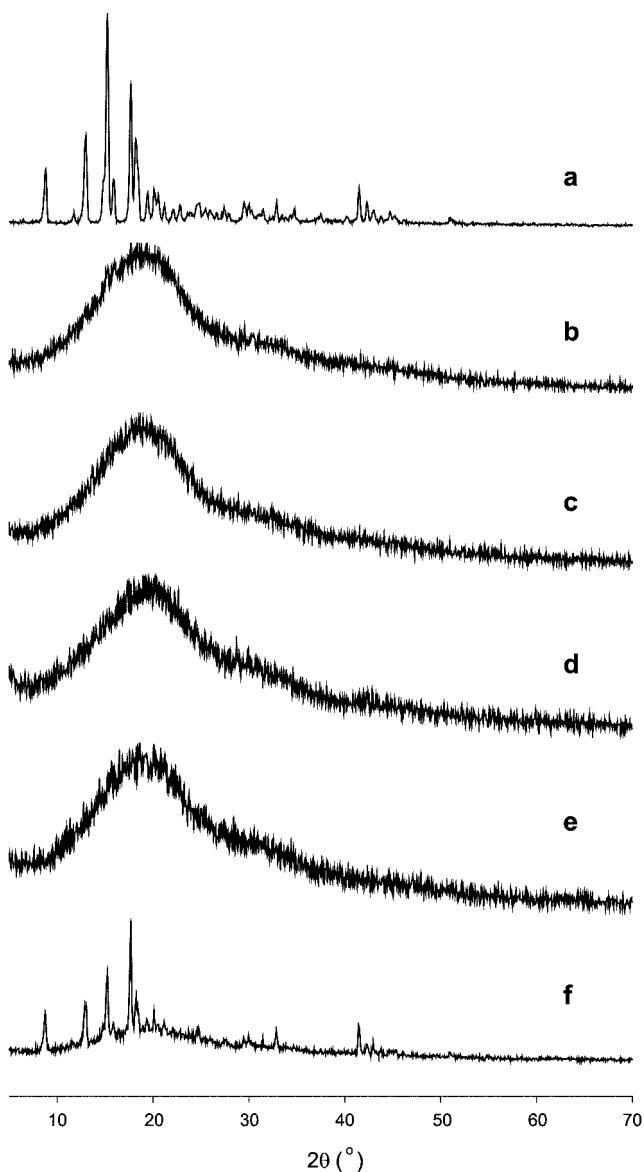
**Figure 3.** X-ray powder diffraction spectra of surfactant-free PLGA nanoparticles. (a) TST, (b) empty nanoparticles, (c) TST-entrapped nanoparticles prepared from DMF by dialysis, (d) TST-entrapped nanoparticles prepared from acetone by dialysis, (e) TST-entrapped nanoparticles prepared from acetone by solvent diffusion method, (f) physical mixture of TST and empty PLGA nanoparticles (prepared by solvent diffusion using acetone, weight ratio of TST : empty nanoparticle = 1.5 : 10).
