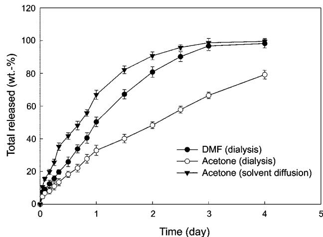
**Figure 4.** Drug release from surfactant-free nanoparticles of poly(DL-lactide-co-glycolide).
