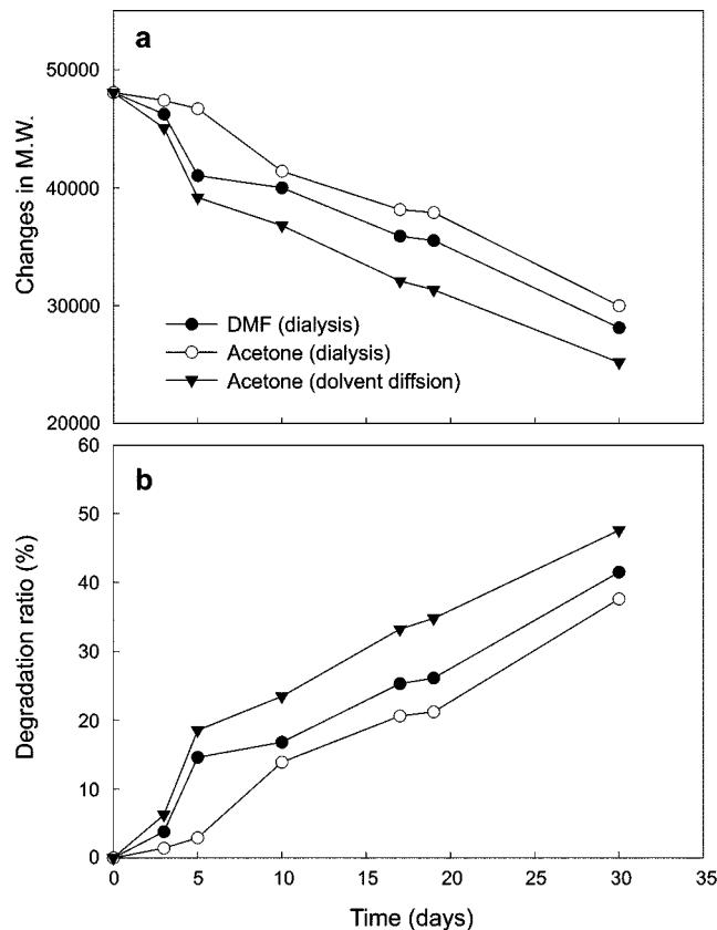
**Figure 5.** *In vitro* degradation profiles of surfactant-free nanoparticles of PLGA. Changes in M<sub>w</sub> (a) and degradation ratio (b). Equation of degradation ratio was described in Experimental part.
