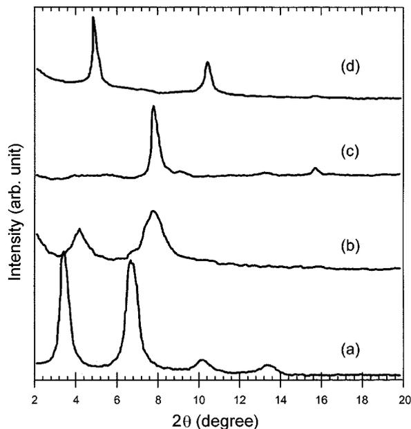
**Figure 1.** Powder XRD patterns for as-prepared  $[C_{60}(C_2H_8N_2)_6]_x-FeOCl$  (a), heat-treated  $[C_{60}(C_2H_8N_2)_6]_xFeOCl$  at 75 °C for 10h (b),  $C_2H_8N_2$ -intercalated FeOCl (c), and DMSO-intercalated FeOCl (d).
