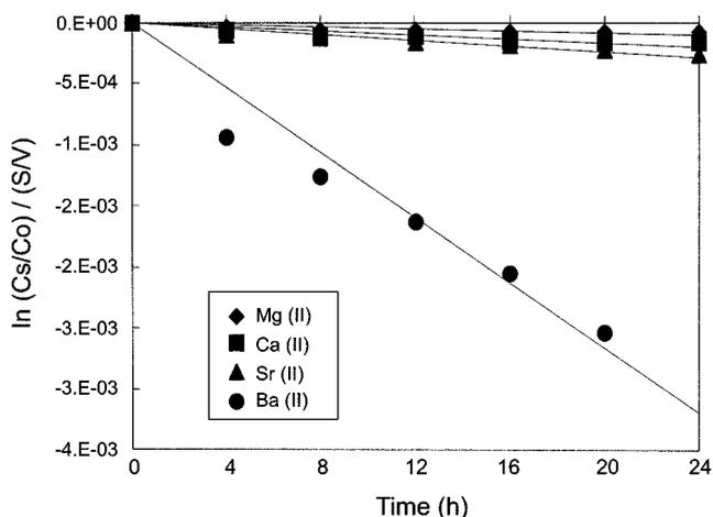
**Figure 2.** Kinetic plot of the permeability for alkaline-earth metal ions as a function of time (h) through a PIM. Source phase: aqueous solution of 10 mM metal nitrate; membrane phase: CTA membrane; [carrier] = 1.0 mM; receiving phase: deionized water.
