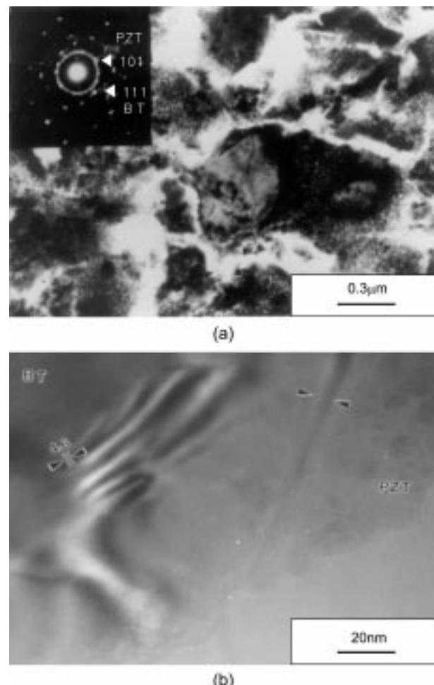
**Figure 9.** TEM image and diffraction pattern of BT seeded PZT powders. (a) low magnification image with diffraction pattern; (b) high magnification image of the interface between BT seed and PZT.
