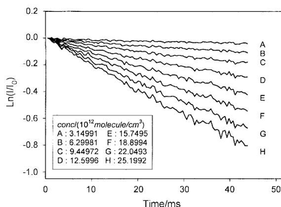
Figure 3. Plot of  $\ln(I/I_0)$  versus reaction time at different concentrations of ethylene at 298 K. The O(<sup>3</sup>P) atom decay rates,  $k_{decay}$ , were obtained from the slope of this plot.
