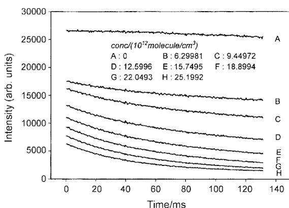
Figure 2. Decay signals of the NO<sub>2</sub> chemiluminescence for the reactions of O(<sup>3</sup>P) atom with various C<sub>2</sub>H<sub>4</sub> concentrations. Without sample, the chemiluminescence intensity is nearly constant over the entire reaction zone as plotted in A.
