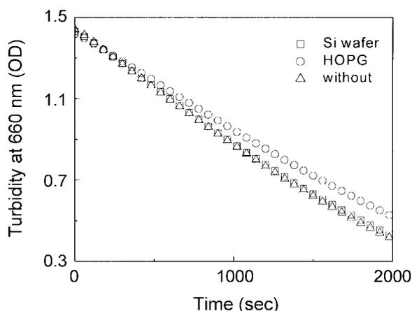
**Figure 2.** Turbidity profiles of PHB granule-suspended solutions at 37 °C by an extracellular PHB depolymerase purified from *A. faecalis* T1.
