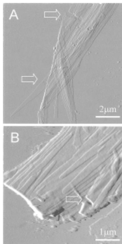
**Figure 3.** AFM topographic images of solution-grown crystals after hydrolysis at room temperature by an extracellular PHB depolymerase purified from *A. faecalis* T1 (A) and 0.1 N NaOH solution (B). The arrows indicate the breakup of lamellar crystals along the *b* axis.
