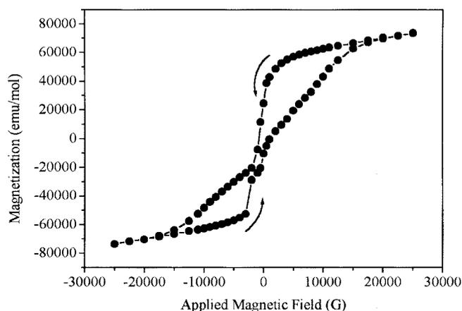
**Figure 7.** Magnetic hysteresis loop of  $\text{Mn}_{12}$ -stearate at 2 K.
