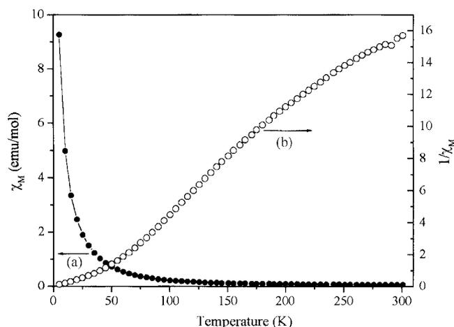
Figure 5. (a) Magnetic susceptibility of Mn<sub>12</sub>-stearate, (b) reciprocal magnetic susceptibility  $\chi_M$  versus temperature of Mn<sub>12</sub>-stearate at 100 Gauss.
