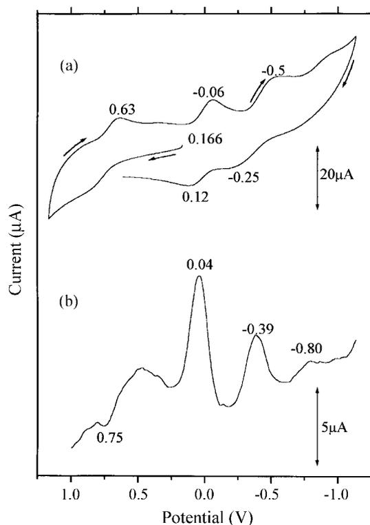
Figure 4. (a) The CV and (b) the DPV data of Mn<sub>12</sub>-stearate.
