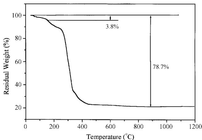
Figure 3. TGA of Mn<sub>12</sub>-stearate under N<sub>2</sub> flowing.
