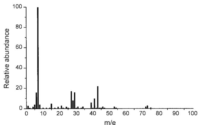
**Figure 9.** The mass spectrum of the film formed on the gold electrode. The eight voltage scans were made between 2.4 and 0.5 V and the number of SIMS scans was 10 with the  $\text{Cs}^+$  beam energy of 100 eV.
