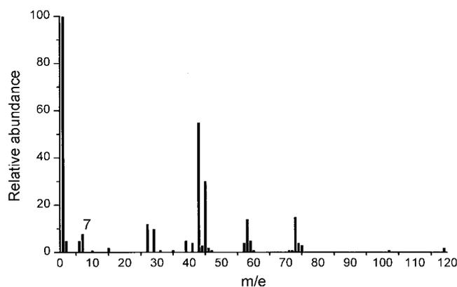
**Figure 8.** The mass spectrum of the film formed on the gold electrode. The potential scan range was between 2.4 V and 1.2 V at an Au electrode, the number of the voltage scan was 6, the energy of the incident  $\text{Cs}^+$  ion beam was 30 eV, and the number of SIMS scan was 23.
