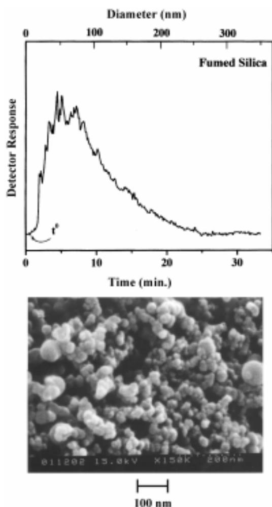
**Figure 8.** Separation of fumed silica sample by FI-AFIFFF along with the SEM micrograph of the original sample. Run condition is the same as used in Figure 7.
