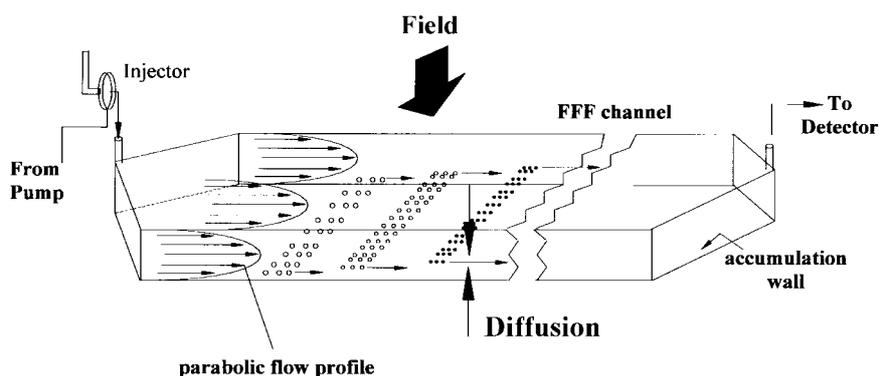
**Figure 1.** Schematic diagram showing parabolic flow streamlines in a rectangular FFF channel. Real sample bands should be more like a distributed form of sample clouds though they appear as discrete sample layers in the diagram.
