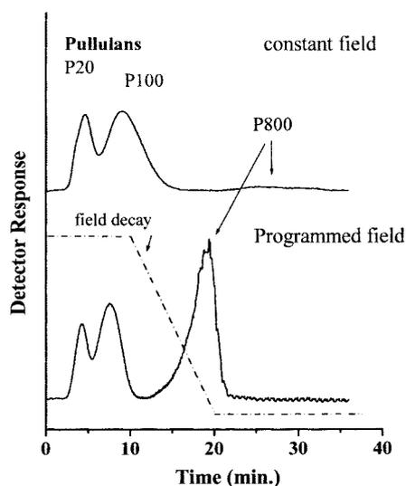
**Figure 10.** Separation of pullulan standards with constant field operation and with linear field programming by FI-AFIFFF obtained at  $\dot{V}_s = \dot{V}_{out} = 0.10$  mL/min. Outflow rate for both runs are the same as  $\dot{V}_{out} = 0.10$  mL/min. For the constant field run,  $\dot{V}_s$  is maintained at 1.20 mL/min. For the programmed run,  $t_1 = 10$  min,  $t_p = 10$  min,  $\dot{V}_{c0} = 1.20$  mL/min,  $\Delta\dot{V}_c = 1.10$  mL/min.
