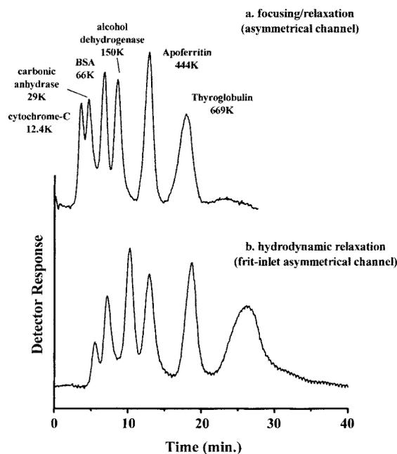
**Figure 9.** Comparison of separation resolution for protein mixtures obtained by (a) a conventional asymmetrical channel and (b) frit-inlet asymmetrical channel. Outflow conditions are fixed as  $\dot{V}_{out} = 0.20$  and  $\dot{V}_c = 7.0$  for both runs. Injection flow rate and the inlet flow rate ( $\dot{V}_{in}$ ) for run a are 0.10 and = 7.10 mL/min. Focusing point is 3.0 cm from the channel inlet. For run b,  $\dot{V}_s = 0.20$ ,  $\dot{V}_f = 7.0$  mL/min.
