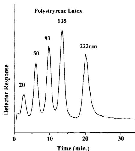
**Figure 7.** Separation of polystyrene latex standards by FI-AFIFFF using hydrodynamic relaxation obtained at  $\dot{V}_s = 0.10$ ,  $\dot{V}_f = 2.5$ ,  $\dot{V}_c = 2.2$ , and  $\dot{V}_{out} = 0.40$  mL/min.
