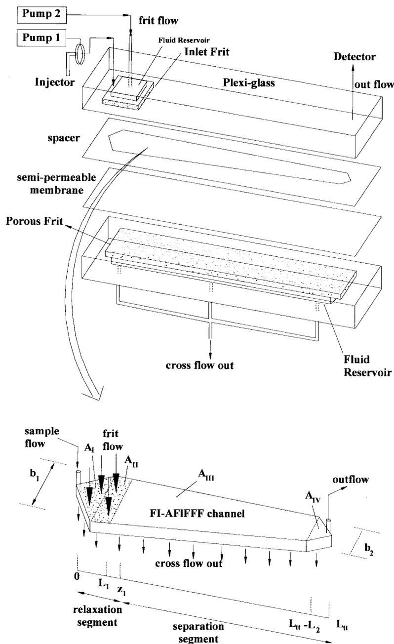
**Figure 3.** Schematic illustration of channel assembly of the frit-inlet asymmetrical flow FFF (FI-AFIFFF) channel. Trapezoidal geometry of channel is enlarged with the two inlet flows (sample and frit flow) and the two outlet flows (crossflow and outflow).
