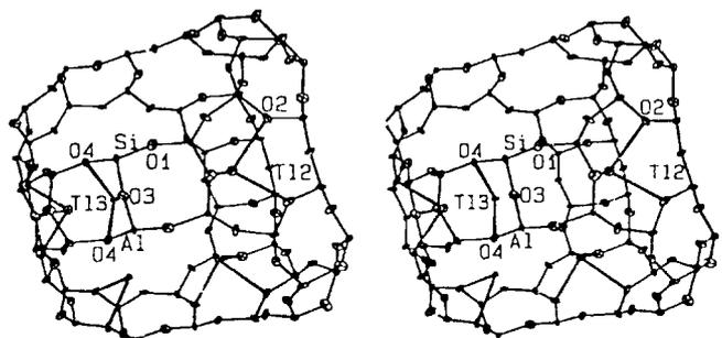
**Figure 5.** Stereoview of the supercage of dehydrated  $\text{Pd}_{21}\text{Tl}_{50}\text{-X}$ . Three  $\text{Tl}^+$  ions at Tl(2) (site II) and two  $\text{Tl}^+$  ions at Tl(3) (site III') are shown. About 50% of supercages can have this arrangement. Ellipsoids of 20% probability are used.
