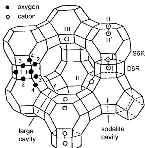
**Figure 1.** A stylized drawing of the framework structure of zeolite X. Near the center of each line segment is an oxygen atom. The numbers from 1 to 4 indicates the different oxygen atoms. Silicon and aluminum atoms alternate at the tetrahedral intersections, except that a silicon atom substitutes for aluminum at about 4% of the Al positions. Extraframework cation positions are labeled with Roman numerals.
