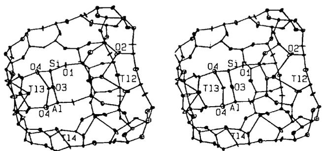
**Figure 3.** Stereoview of the supercage of dehydrated  $\text{Pd}_{18}\text{Tl}_{56}\text{-X}$ . Three  $\text{Tl}^+$  ions at Tl(2) (site II), one  $\text{Tl}^+$  ion at Tl(3) (site III'), and one  $\text{Tl}^+$  ion at Tl(4) (site III') are shown. About 25% of supercages can have this arrangement. Ellipsoids of 20% probability are used.
