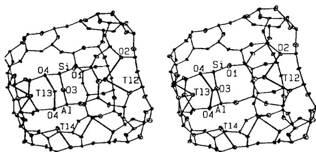
**Figure 6.** Stereoview of the supercage of dehydrated  $\text{Pd}_{21}\text{Tl}_{50}\text{-X}$ . Three  $\text{Tl}^+$  ions at Tl(2) (site II), one  $\text{Tl}^+$  ion at Tl(3) (site III'), and one  $\text{Tl}^+$  ion at Tl(4) (site III') are shown. About 37.5% of supercages can have this arrangement. Ellipsoids of 20% probability are used.
