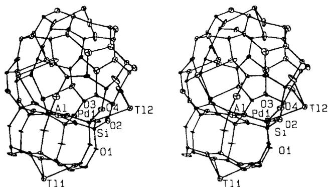
**Figure 2.** Stereoview of a sodalite cavity with an attached D6R in dehydrated  $\text{Pd}_{18}\text{Tl}_{56}\text{-X}$ . Three  $\text{Pd}^{2+}$  ions at Pd(1) (site I'), one  $\text{Tl}^+$  ion at Tl(1) (site I') and four  $\text{Tl}^+$  ions at Tl(2) (site II) are shown. About 25% of sodalite cavities can have this arrangement. Ellipsoids of 20% probability are shown.
