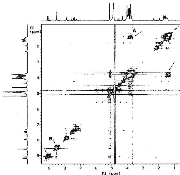
**Figure 3.** 600 MHz ROESY spectrum for  $\alpha$ -CD/2NC<sub>12</sub>V in D<sub>2</sub>O at 25 °C. NOE crosspeaks between spacer alkyl chain and  $\alpha$ -CD are indicated by arrow A, and the exchange crosspeaks in viologen region are indicated by arrow B. [ $\alpha$ -CD] = 1 mM,  $\tau_{\text{mix}}$  = 100 ms were used.
