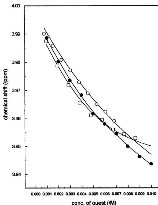
**Figure 2.** Nonlinear least squares fitting of NMR shift of H<sub>3 $\alpha$</sub>  proton of  $\alpha$ -CD caused by complexation with 2NC<sub>n</sub>V in D<sub>2</sub>O at 25 °C. n=3 (○), n=5 (●), n=9 (□).
