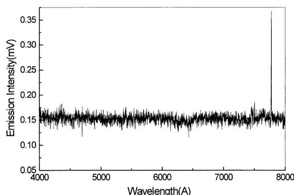
**Figure 4.** Observed emission spectrum for the transition of O(<sup>1</sup>D) to O(<sup>3</sup>P) states generated from pure O<sub>2</sub> gas.
