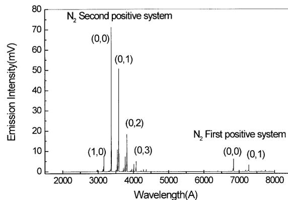
**Figure 3.** Typical N<sub>2</sub> emission spectrum showing the first (C<sup>3</sup>Π<sub>u</sub> → B<sup>3</sup>Π<sub>g</sub>) and the second (B<sup>3</sup>Π<sub>g</sub> → A<sup>3</sup>Σ<sub>u</sub><sup>+</sup>) positive transitions in the range of 200-800 nm wavelength. (v', v'') designates vibrational quantum numbers for higher and lower electronic states, respectively.
