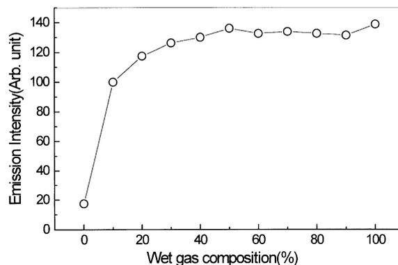
**Figure 6.** The emission intensity of  $\text{OH}(\text{A}^2\Sigma^+)$  radicals generated by corona discharge as a function of the concentration of water vapor within  $\text{N}_2$  gas.
