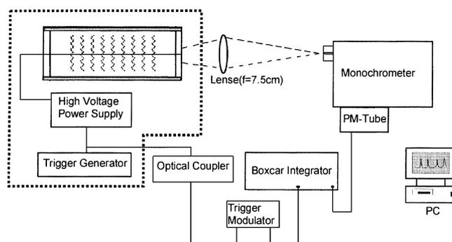
Figure 2. Schematic diagram for the optical emission measurement.
