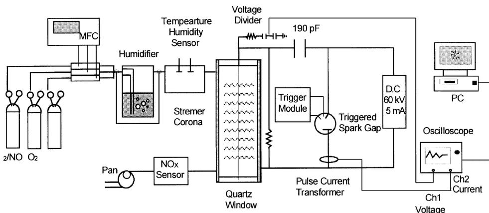
Figure 1. Schematic diagram of corona discharge experimental system.
