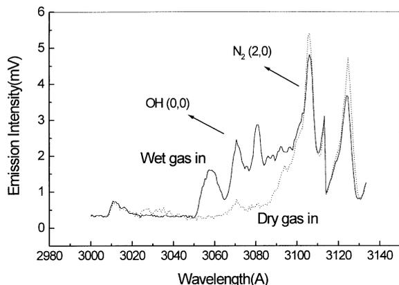
**Figure 5.** Observed  $\text{OH}(\text{A}^2\Sigma^+)$  emission spectra with dry (solid line) and humid (dotted line)  $\text{N}_2$  gas, respectively.
