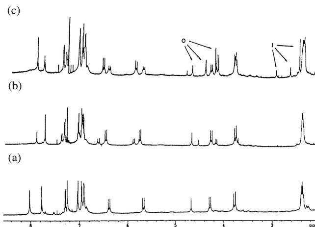
**Figure 11.** The more rigid system 23 and its  $^1\text{H}$  NMR (a) in  $\text{CDCl}_3$ . (b) 0.5 equivalents of 1-adamantane carboxylic acid added. (c) 0.6 equivalents of 1-ferrocenecarboxylic acid added. The signals of the guest inside and outside are labeled with "i" and "o" respectively.
