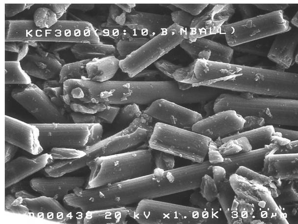
**Figure 5.** SEM image of MPCF3000 electrode.
